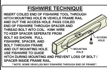
6. Reverse fishwire 7/16-14 x 1 1/2" carriage bolt and SP11 spacer into the drilled access hole in the passenger frame rail (and driver side frame rail if it is a drilled access hole).
