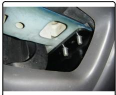
8. Reinstall the (2) screws removed in Step (1) and secure the bumper cover to the radiator support bracket.
