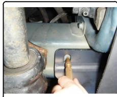
4. Drill holes marked in Step (3). Enlarge the drill hole in the passenger side frame rail to allow 7/16" carriage bolts and SP11 spacers to pass through. **Note:** If existing access hole is not present in driver side frame rail, enlarge the drill hole to allow 7/16" carriage bolts and SP11 spacers to pass through.
