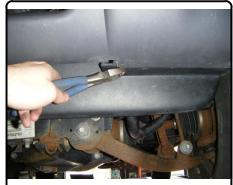
2. Mark and trim the plastic wheel well. **Note:** Dimensions are approximate, confirm fit before trimming.
