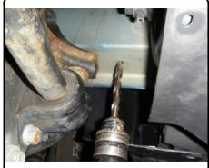
5. Fishwire 7/16-14 x 1 1/2" carriage bolts and SP11 spacers through the access holes and out the (3) holes in the drivers side frame rail ((2) holes if it is a drilled access hole) and (2) holes in the passenger side frame rail. (See Fishwire Technique)
